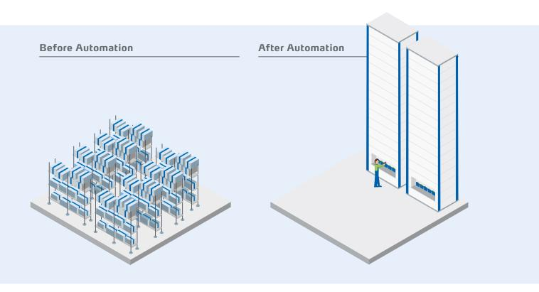
Implementing an automated solution immediately reduces the amount of square footage required to store items within static shelving and pallet rack in two ways: one, by utilizing previously unused overhead space, and two, by compressing items stored within the technology for greater storage capacity. This is because the volumetric efficiency of each automated technology is so much greater, shown below.
