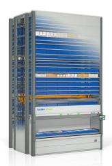
Vertical Lift Modules (VLMs) – An enclosed automated storage and retrieval system that incorporates two columns of trays with a central inserter/extractor that automatically locates and retrieves stored trays from both columns, then presents them to the operator at a waisthigh pick window. These systems save up to 85% of floor space compared to static shelving and rack.
