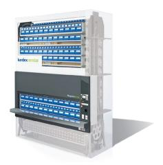
Vertical Carousels – Comprised of a series of shelves that rotate around a track—similar to a Ferris wheel—these automated storage and retrieval systems quickly deliver stored items to an ergonomically positioned work counter at the operator's command. When compared to static shelving and rack, they save up to 75% of floor space.
