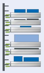
Similarly, carriers within a vertical carousel can be fitted with shelves and drawers to provide the exact storage heights your product mix requires. When compared to wasted capacity within manual shelving, these automated systems recover a tremendous amount of capacity.
