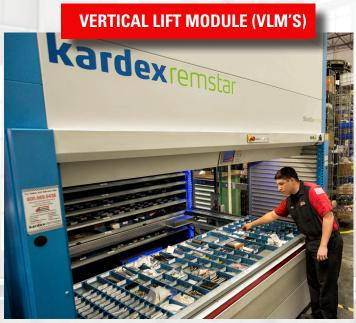
VLM's are perfect for variable or changing part sizes. They can save up to 85% of floor space by utilizing full ceiling height, the dynamic shelving maximizes storage density and improves ergonomics with goods-to-person delivery.
