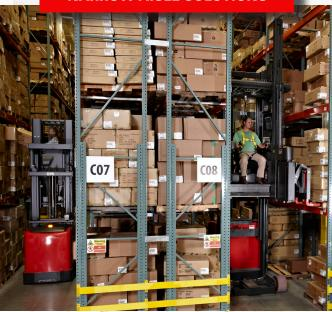
Grow vertically without expanding horizontally, Raymond's narrow aisle trucks can operate in aisles that are less than half the width required by conventional forklifts, with a greater stack height capability.
