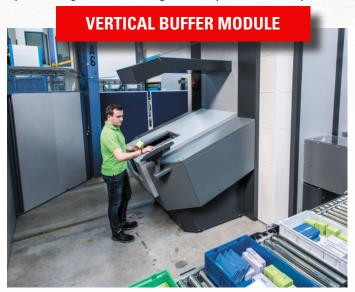
The LR35 vertical buffer module has been designed to meet a broad range of storage and retrieval applications including buffering, kitting, and order picking.
