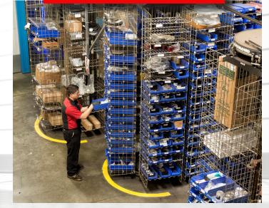
Horizontal carousels offer affordable, reliable storage plus high-speed picking performance. They have fast access times for increased productivity and save up to 60% of floor space by eliminating wasted aisle space.
