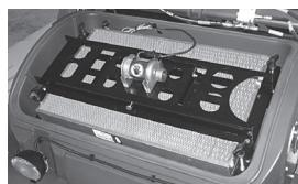
Ultra-Web® dust filter is >98% efficient on 0.3 - 1 micron dust. All dust is locked in the hopper behind only 1 critical seal incorporated in the dust filter. Captured dust is shaken directly back into the hopper.
