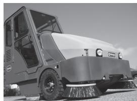
The optional all weather cab keeps the operator comfortable and productive. Clear-View™ window in the cab provides a safe view of the right side broom.
